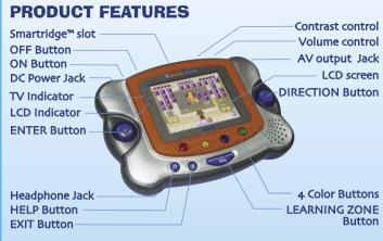
"ON" Button Press this button to turn the unit ON.
